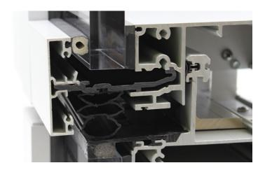
A continuous polyamide thermal break applied vertically and horizontally helps provide ultra-thermal performance levels. Extruded polymer inserts allow a great deal of flexibility – changing the depth of the infill from a double insulating glass unit (IGU) to a triple IGU is as easy as changing the depth of the thermal separator. Depending on the depth of the separator and IGU type, the performance can be thermal, high-thermal or ultra-thermal.
