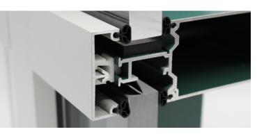
Engineered polymer clips are placed intermittently to separate the face and gutter of low-rise curtain walls and other framing systems. The clip eliminates contact between exterior and interior aluminum so that the transfer of heat is reduced from the inside to the outside or vice versa. The interior-exterior separation also helps prevent interior condensation.
