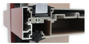
The patented IsoStrut® Thermal Break method achieves a highstrength bond between the aluminum and the thermal break material, which creates a composite assembly suitable for use in monumental curtain walls.
