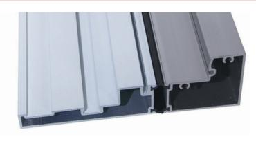
To improve the U-factor and CRF, the IsoWeb® thermal break system consists of two parallel glass-reinforced nylon strips installed continuously along the length of the extrusion. The depth of the thermal break can accommodate standard insulating infills of 1" thick or it can be increased to accept high-performance, triple-sealed insulating units
